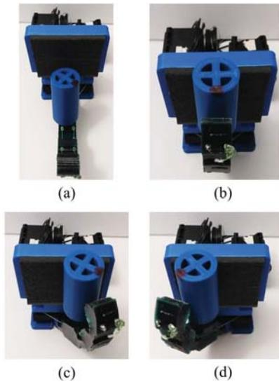
Fig. 10. The anthropomorphic finger performing a manipulation task. (a) The adaptive finger with the cylindrical object. (b) Initial grasping position. (c) Rolling clockwise  $45^\circ$ . (d) Rolling counterclockwise  $90^\circ$ .
