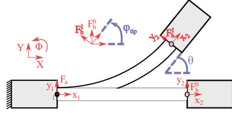
Fig. 5. A flexure joint with straight curvature,  $\kappa = 0$ . One link is fixed at inertial frame  $\mathcal{F}_a$  while the other link performs a planar motion with a body-fixed frame  $\mathcal{F}_b$ . The flexure tip angle  $\varphi_{\text{tip}}$ , described by the rotation of body-fixed frame  $\mathcal{F}_b$ , is equal with the joint angle  $\theta$ .
