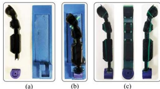
Fig. 6. The fabrication process of the developed finger. (a) The reusable mold in blue, the rotating base in purple, and the sacrificial mold in black. (b) The elastomer material at the curing phase. (c) Side views and front view of the fabricated finger.
