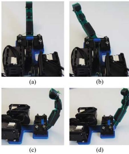
Fig. 9. The anthropomorphic finger in various configurations. (a) Finger in the neutral (rest) position. (b) Finger abduction achieved by using the corresponding tendon-driven system. (c) Finger flexion without any abduction. (d) Finger flexion in an abducted angle.
